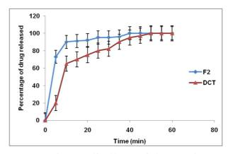
Fig.3: Dissolution profile of furosemide from F2 and DCT (values represent mean±SD, n=3), DCT: direct conventional tablet
