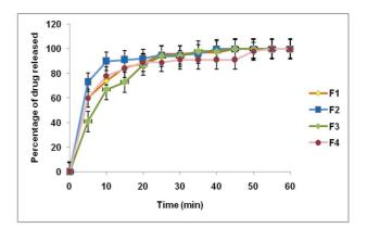
Fig. 2: Dissolution profile of furosemide from liquisolid tablets (values represent mean±SD, n=3)
