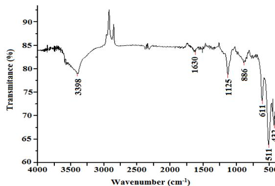
Fig. 2: FT-IR spectrum of CuO nanoparticles
