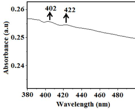
Fig. 3: Optical absorption spectrum of CuO nanoparticles
