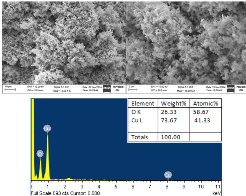
Fig. 4: a. SEM images of CuO nanoparticles, b. Energy dispersive spectrum of CuO nanoparticles
