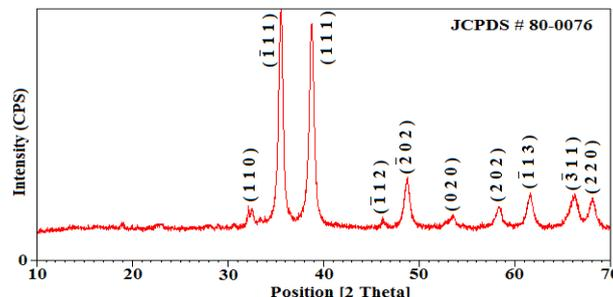
Fig. 1: X-ray diffraction patterns of CuO nanoparticles
