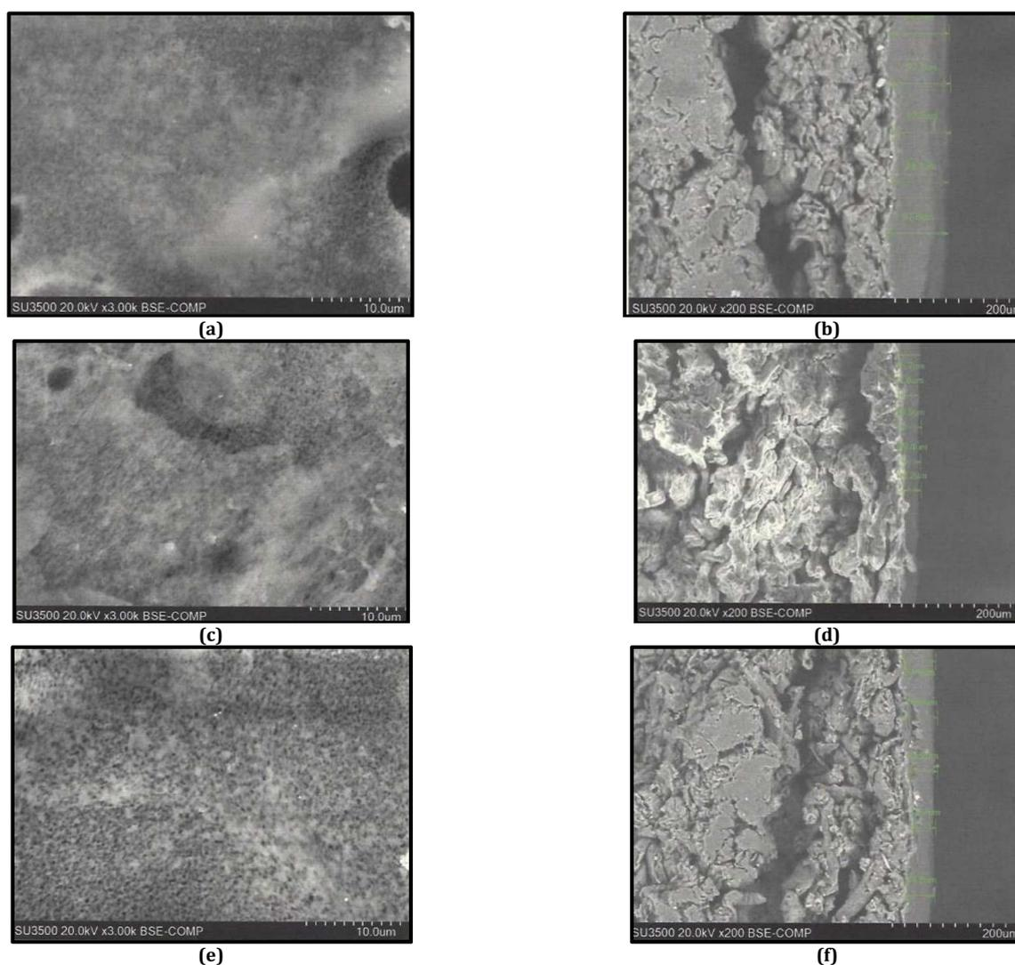
**Fig. 1: Scanning electron microscope result for film coated surface with 3000x magnification (left) and thickness of coating layer with 200x magnification (right): FA (a,d), FB (b,e), and FC (c,f)**
