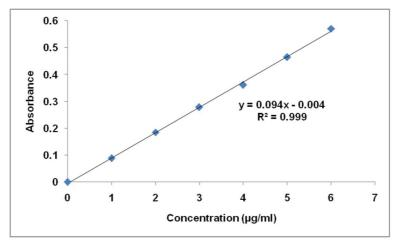
Fig. 2: Calibration curve of ciprofloxacin HCl in 0.1 N HCl
