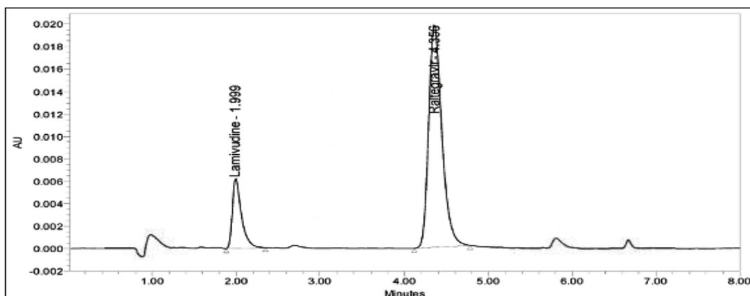
**Fig. 6: Acid degradation of LAM and RAL**
