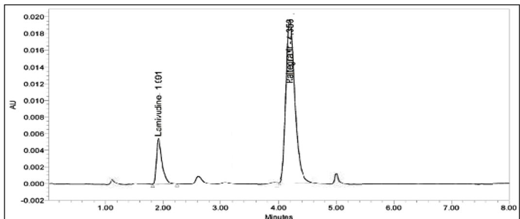
Fig. 9: Photolytic degradation of LAM and RAL
