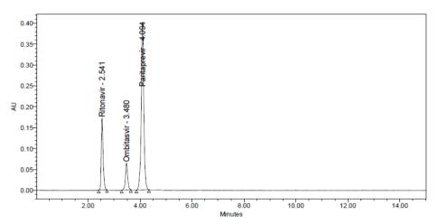
Fig. 36: Chromatogram for peroxide degradation
