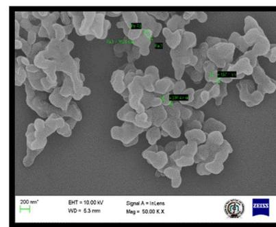
**Fig. 6: SEM image of catechin nanoformulation with surface morphology**
