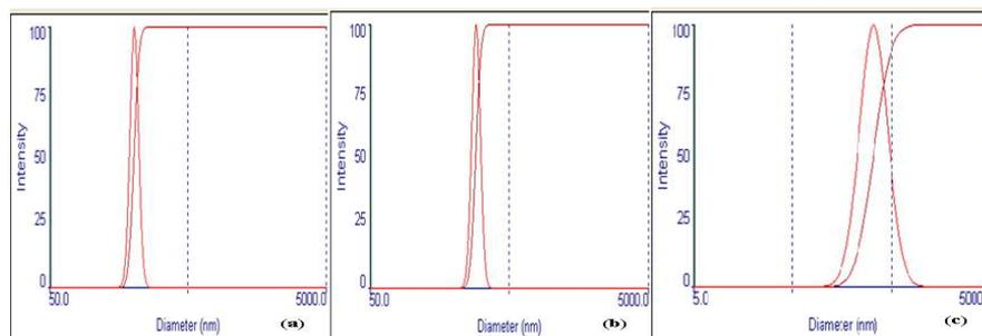
**Fig. 7: Particle size distribution of NF1 (a), NF2 (b) and NF3 (c)**
