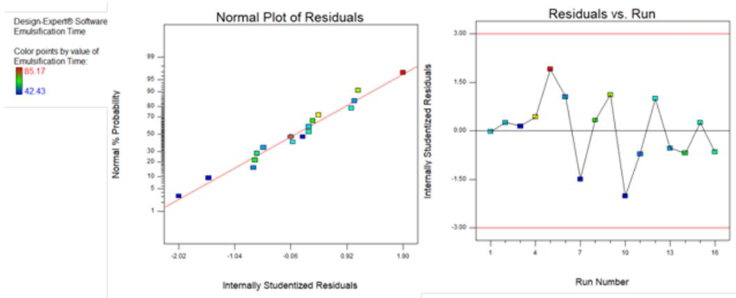
Fig. 1: The normal probability plot residual of emulsification time
