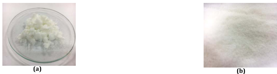
Fig. 4: \alpha -cellulose of kapok pericarpium before hydrolyzed (a) and MCC of kapok pericarpium (b)
