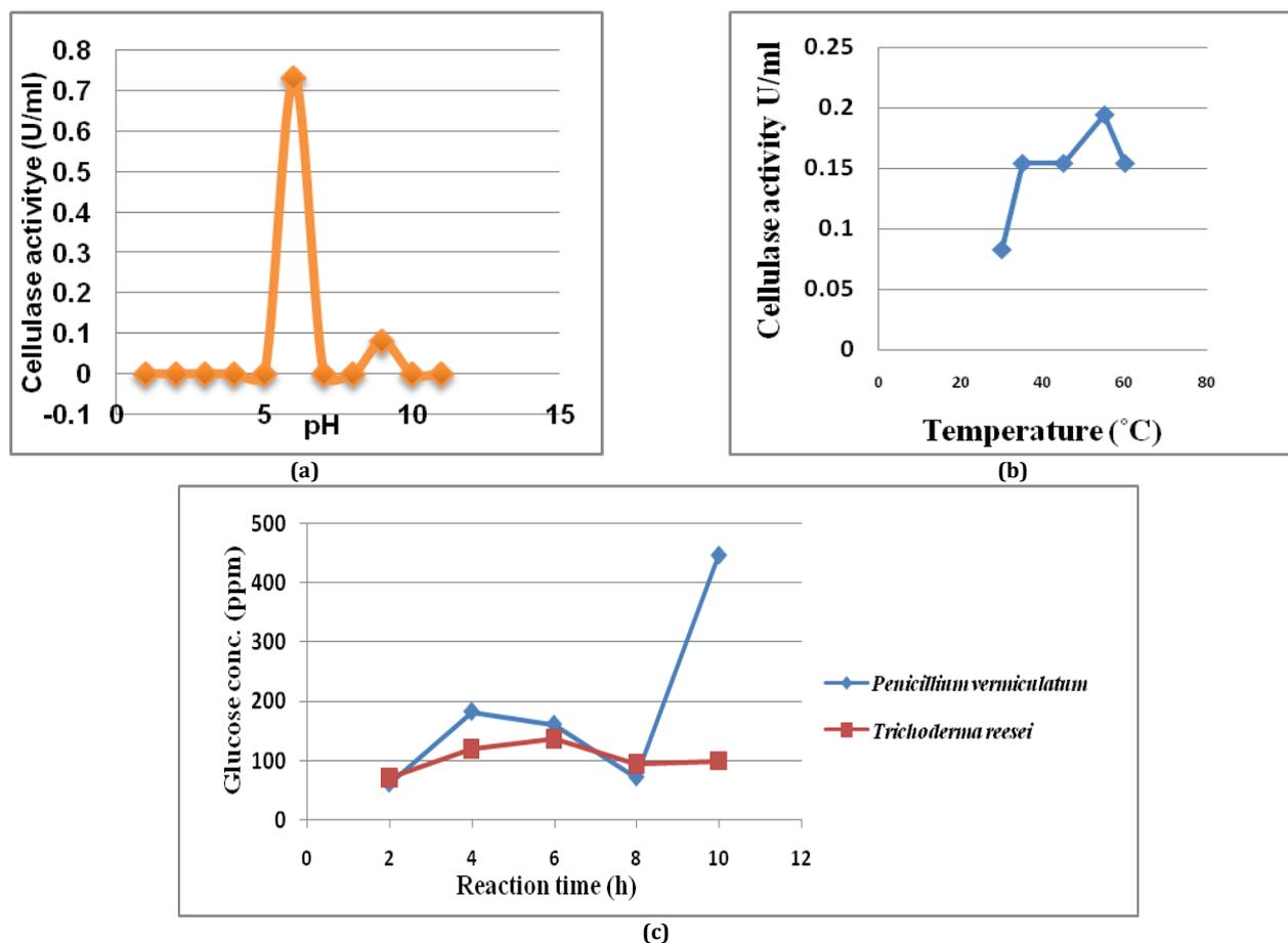
Fig. 3: Effect of pH on the cellulase activity of *Penicillium vermiculatum* (a), the effect of temperature on the cellulase activity of *Penicillium vermiculatum* (b), and the optimization duration of hydrolysis (c)
