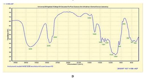
Fig. 6: FTIR spectrum of the selected formula F10 [A], Naproxen [B], carbomer CB [C], and HPMC K100 [D]
