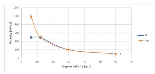
Fig. 2: The viscosity versus angular velocity for F7 (HPMC K40) and F10(HPMC K100) for the same concentration of CB (0.7%) at room temperature (n=3)
