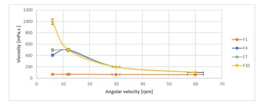
Fig. 1a: The viscosity of naproxen ocular in-situ gel formulas at 0.75% of the hydrophilic polymer, in relation to the angular velocity at room temperature (n=3)
