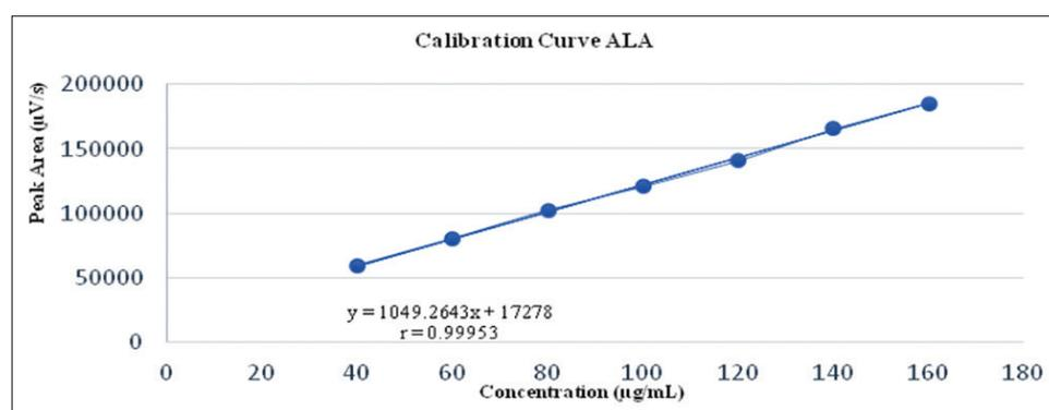
Fig. 2: Alpha-linolenic acid calibration curve
