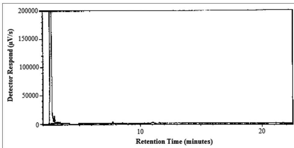
Fig. 1: Results of esterification chromatograms of blanco sample without addition of standard alpha-linolenic acid and docosahexaenoic acid
