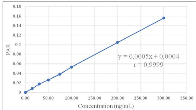
**Fig. 2: Methamphetamine calibration curve**
