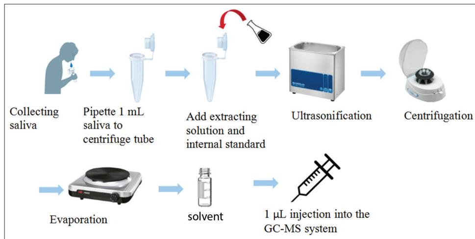
**Fig. 1: Working scheme of salivary sample preparation**
