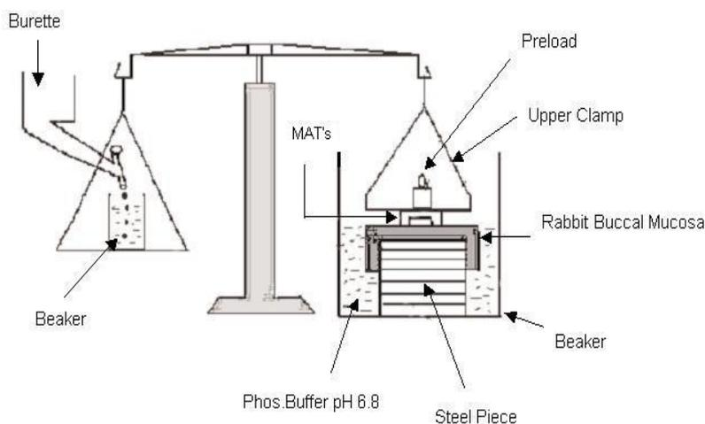
**Fig. 1: Mucoadhesive strength measurement apparatus [19]**
