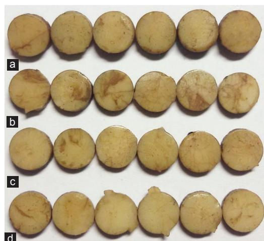
**Fig. 2.** Nanoionomer specimens after immersion in a coffee-based solution: (a) Unpolished nanoionomer; (b) nanoionomer polished using Sof-Lex XT Superfine; (c) nanoionomer polished using PoGo; and (d) nanoionomer polished using OptraPol
