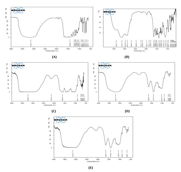
Fig. 3: FTIR Spectra: (A) Telmisartan (B) JFS2 (C) CCS (D) F5 (E) F11, JFS2-Jack fruit seed starch extracted by 0.1% sodium hydroxide; CCS-Croscarmellose sodium; F5-FDT of Telmisartan with JFS2; F11-FDT of Telmisartan with CCS
