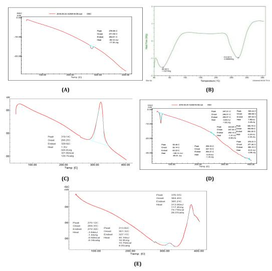
Fig. 4: DSC Thermograms: (A) Telmisartan (B) JFS2 (C) CCS (D) F5 (E) F11; JFS2–Jack fruit seed starch extracted by 0.1% sodium hydroxide; CCS–Croscarmellose sodium; F5–FDT of Telmisartan with JFS2; F11–FDT of Telmisartan with CCS
