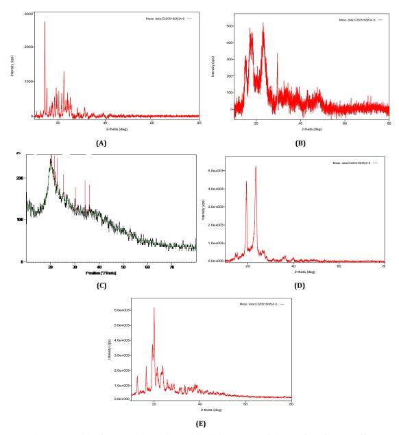
Fig. 6: X-Ray Diffractograms: (A) Telmisartan (B) JFS2 (C) CCS (D) F5 (E) F11; JFS2–Jack fruit seed starch extracted by 0.1% sodium hydroxide; CCS–Croscarmellose sodium; F5–FDT of Telmisartan with JFS2; F11–FDT of Telmisartan with CCS
