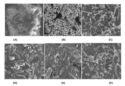
Fig. 5: SEM Images: (A) Jack fruit raw seed powder (B) JFS2 (C) Telmisartan, (D) CCS (E) A blend of Telmisartan and JFS2 (F) A blend of Telmisartan and CCS; JFS2–Jack fruit seed starch extracted by 0.1% sodium hydroxide; CCS–Croscarmellose sodium
