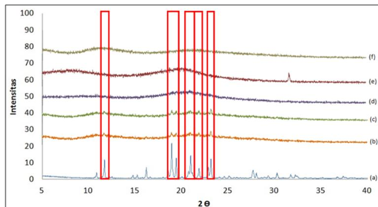
Fig. 3: PXRD result of glibenclamide (a), F1 (b), F10 (c), F19 (d), HPMC (e), PVP (f)
