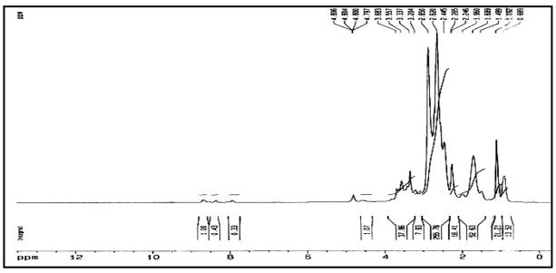
Fig. 5: NMR Spectra of 5.0G PPI dendrimer
