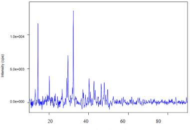
Fig. 4: XRD pattern of synthesized FeNPs
