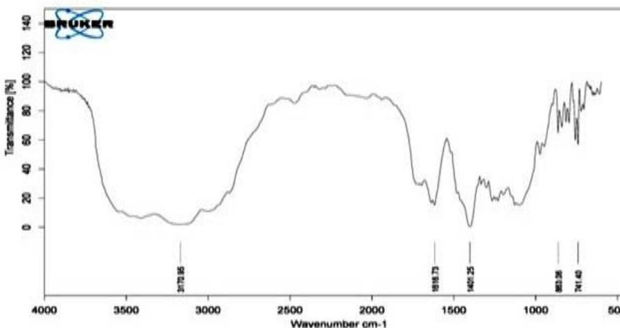
**Fig. 5: FTIR spectra of optimized solid dispersion (TS5)**
