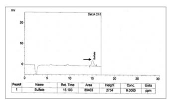
Fig. 1: Ashing-water digestion ion chromatogram of crude sulfated polysaccharide of *Codium edule* showing the presence of sulfate with a retention time of 15 min and an area of 89,403 mAu
