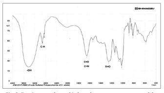
Fig. 2: Fourier-transformed infrared spectroscopy spectra of the crude sulfated polysaccharide of *Codium edule* showing present functional groups in the algal sample
