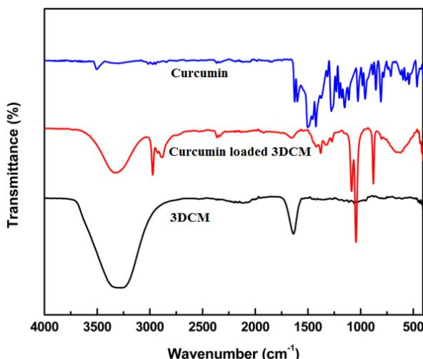
**Fig. 4: FTIR spectra of pure curcumin, pure 3DCM and optimized curcumin loaded 3DCM**
