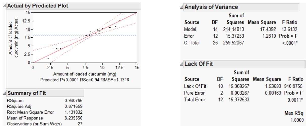
**Fig. 1: Actual versus predicted profile, analysis of variance and lack of fit for the response amount of loaded curcumin into 3DCM****Table 3: The parameter estimates for the response amount of loaded curcumin into 3DCM**
