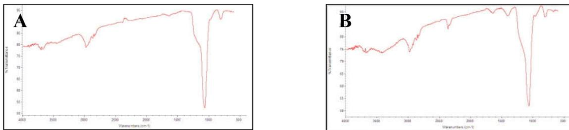
Fig. 3: FTIR spectra of (A) silica-based mesoporous MCM and (B) boron-silica based mesoporous BMCM
