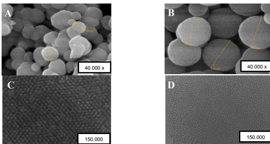
Fig. 2: SEM image of (A) silica-based mesoporous MCM and (B) boron-silica based mesoporous BMCM and TEM image of (C) silica-based mesoporous MCM and (D) boron-silica based mesoporous BMCM
