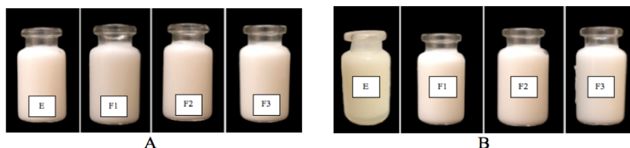
Fig. 1: Appearance of EVOO emulsion (E) and liquid crystal emulsions (F1, F2, F3) (A: Before storage. B: After storage for 12 w at room temperature)
