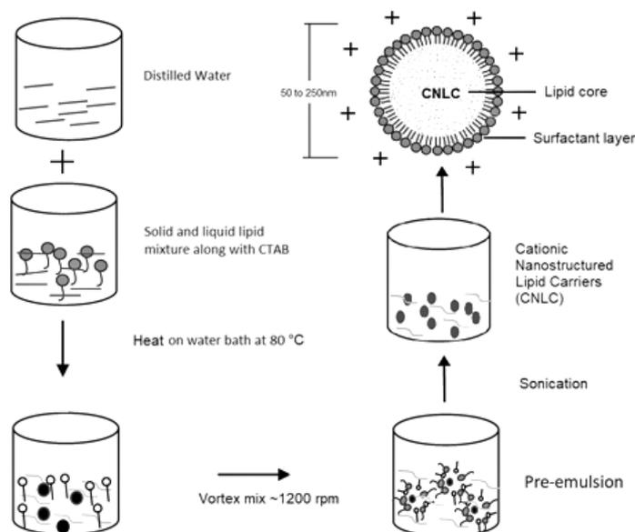
Fig. 1: Method of preparation for CNLC
