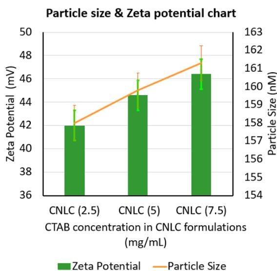
Fig. 3: Graph showing particle size and zeta potential of various CNLC formulations (n=3)
