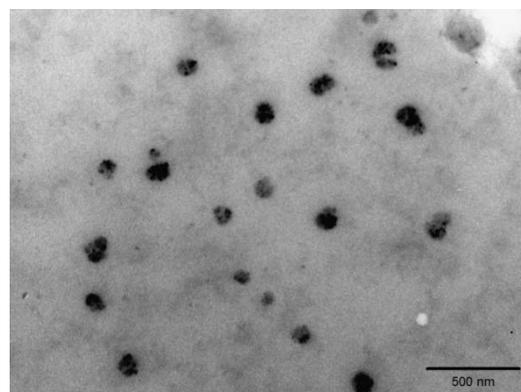
Fig. 8: Transmission electron microscopy (TEM) image for rhodamine optimum CNLC formulation
