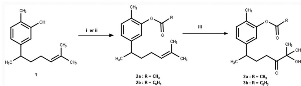
**Fig. 1: Structures and synthetic routes of xanthorrhizol derivatives. Reaction conditions: (i) Acetic anhydride NaHCO<sub>3</sub>, ethyl acetate, rt; (ii) benzoyl chloride, NaOH, cold (0°C–5°C); and (iii) KMnO<sub>4</sub>, acetic acid, acetone, water, 0°C–5°C**
