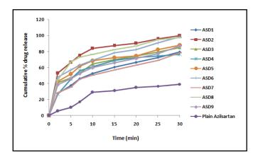
Fig. 3: Cumulative % drug release of Azilsartan Solid Dispersion tablets compared with plain azilsartan (All value represents mean±SD (n=3))
