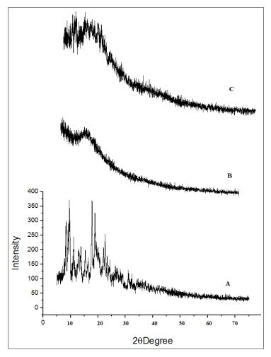
Fig. 6: XRD of A: Azilsartan, B: Soluplus, C: Formulation ASD-2
