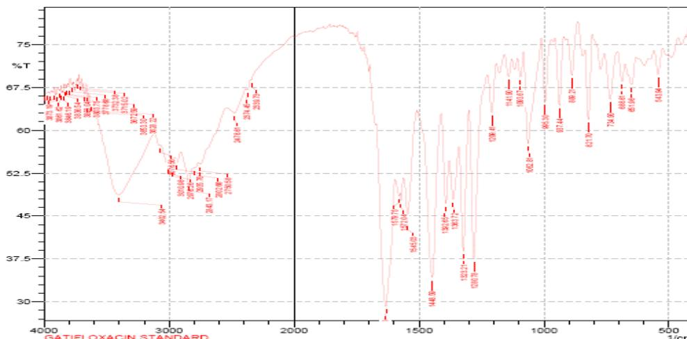
Fig. 2: FTIR spectrum of gatifloxacin drug sample
