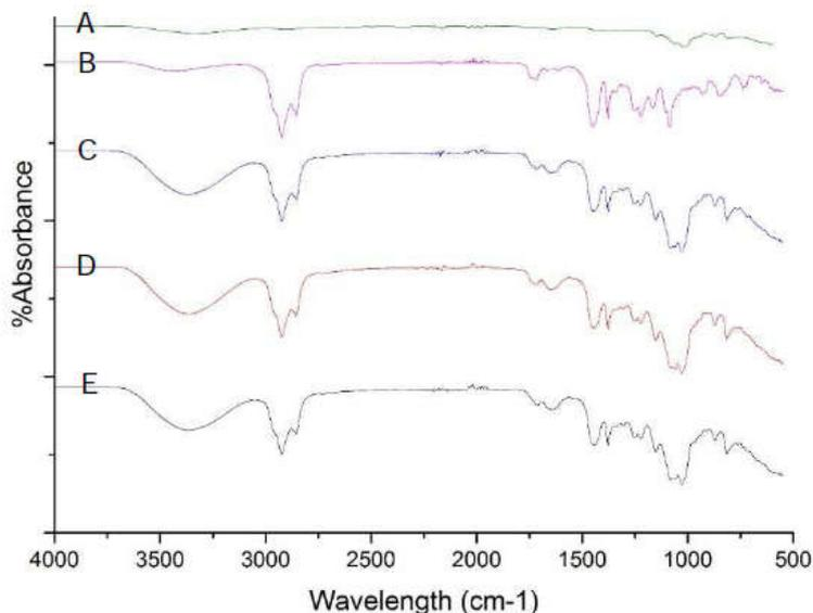
**Fig. 4: Spectra FT-IR of (A) aerogel; (B) vitamin E; (C) aerogel from APE type 1+vitamin E; (D) aerogel from APE type 2+vitamin E; and (E) aerogel from APE type 3+vitamin E, APE: *Arenga pinnata* endosperm**
