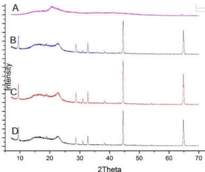
**Fig. 6: X-RD spectra of (A) aerogel from APE type 2; (B) aerogel from APE type 1+vitamin E; (C) aerogel from APE type 2+vitamin E; and (D) aerogel from APE type 3+vitamin E, APE: *Arenga pinnata* endosperm**
