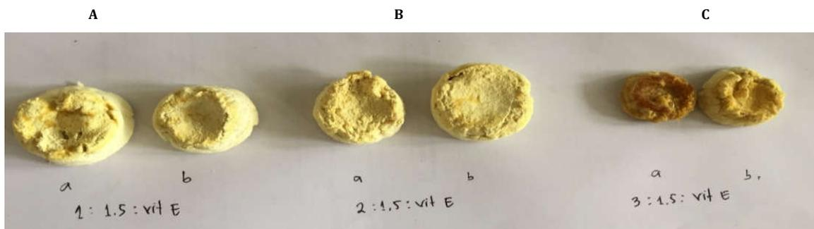
Fig. 9: The images of (A) aerogel from APE type 1+vitamin E; (B) aerogel from APE type 2+vitamin E; and (C) aerogel from APE type 3+vitamin E, APE: *Arenga pinnata* endosperm
