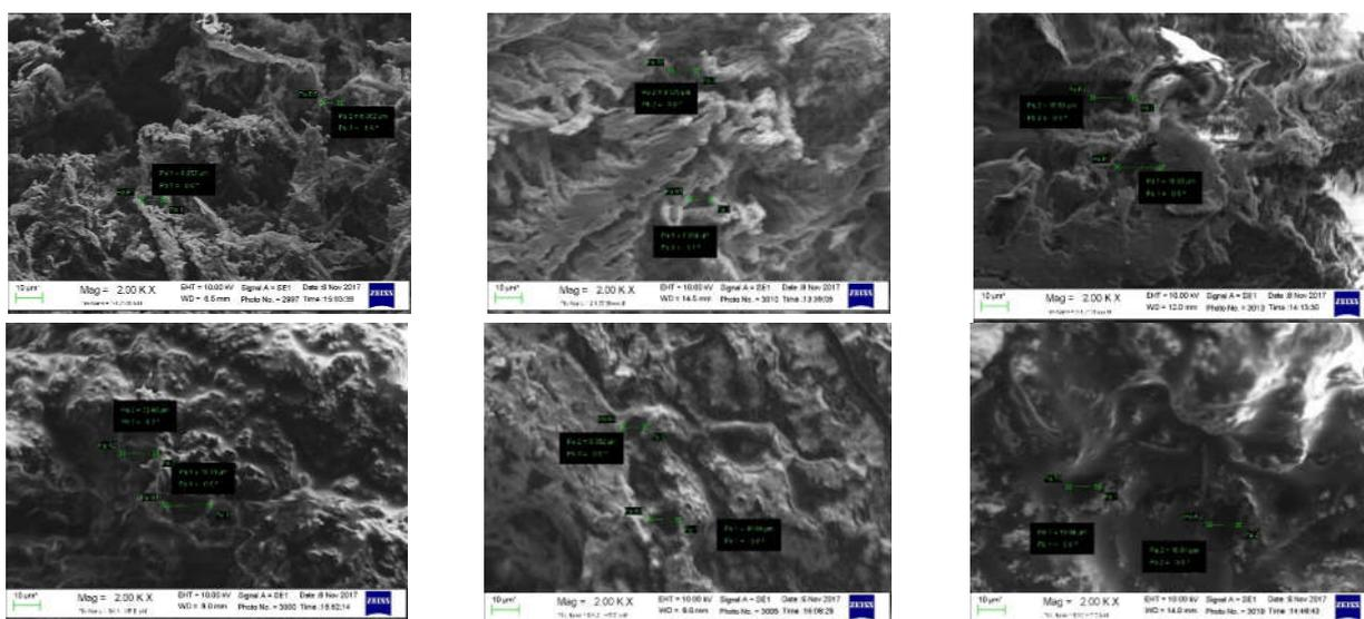
**Fig. 5: SEM images of (A-C) aerogel from APE type 1-3 concentration of 1.25% and (D-F) aerogel from APE type 1-3 concentration of 1.5%+vitamin E in solvent exchange time of 36 h, APE: *Arenga pinnata* endosperm**
