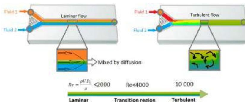
Fig. 6: Laminar and turbulent flow in microfluidic system [63]
