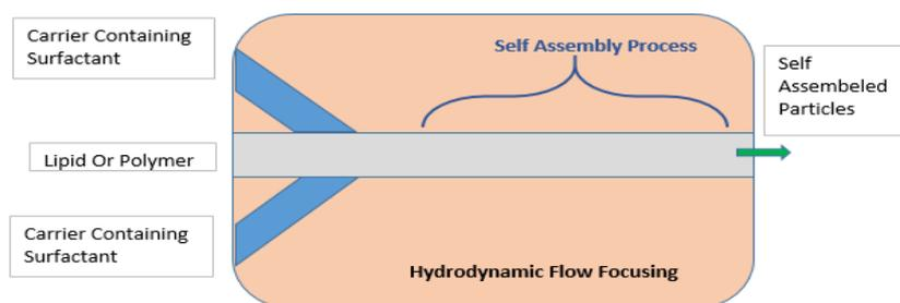
Fig. 1: Hydroderma flow micromixer for the fabrication of microfluidic drug carriers [12]
