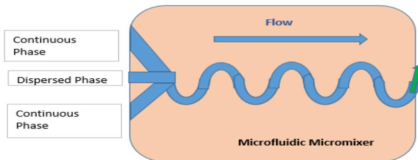
Fig. 2: Simple microfluidic mixer for the fabrication of microfluidic drug carriers [12]
