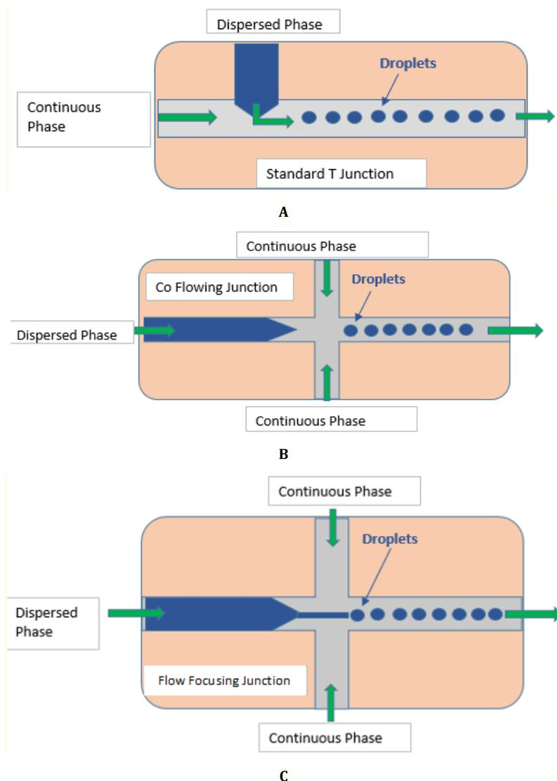
Fig. 4: Droplets microfluidic platforms (A) T-junction; (B) co-flowing junction and (C) flow-focusing junction [12]
