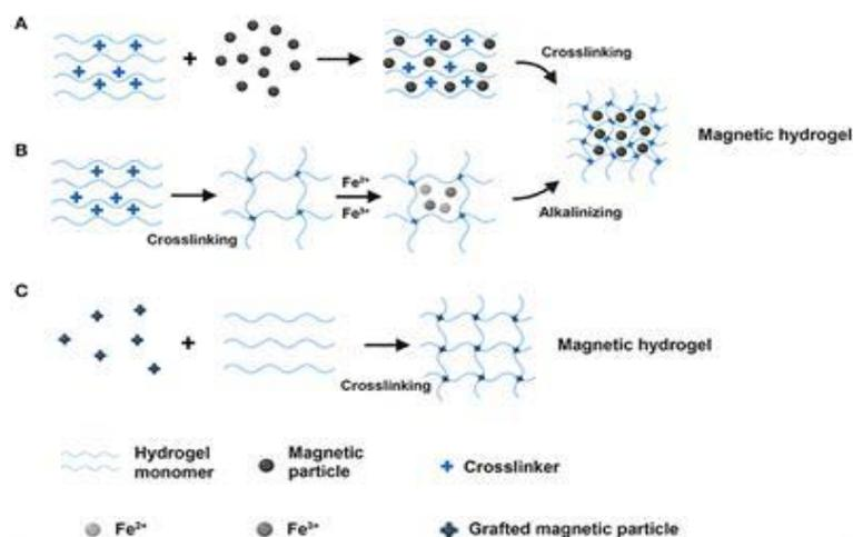
Fig. 4: The schematic diagram of the main three routes for the synthesis of the magnetic hydrogels. (A) The blending method. (B) The in situ precipitation method. (C) The grafting-onto method [42]
