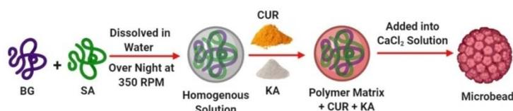
Scheme 1: Schematic procedure for the preparation of CUR encapsulated SA/BG/KA microbeads
