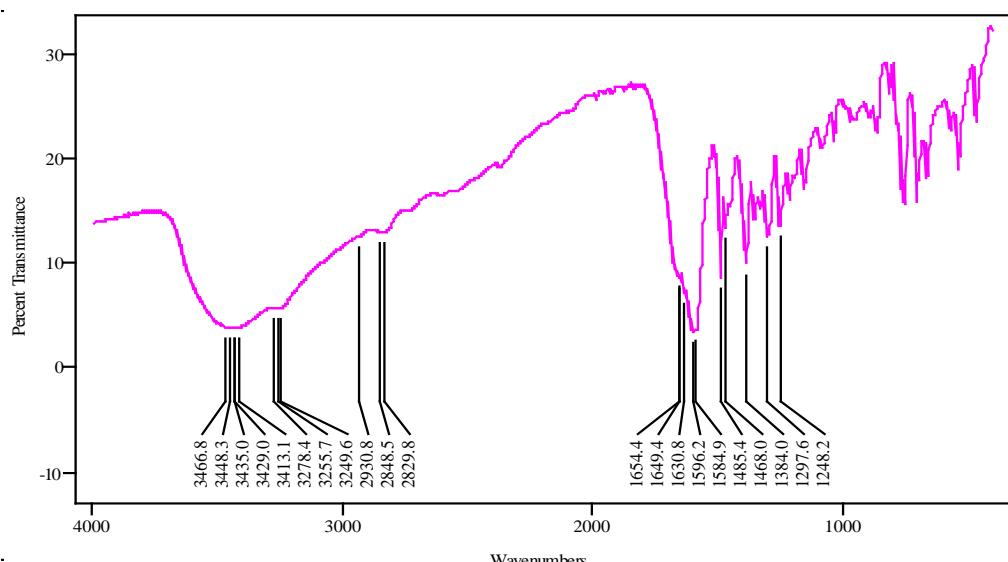
**Fig. 4: FT-IR spectra of ASA-valine cocrystal**
