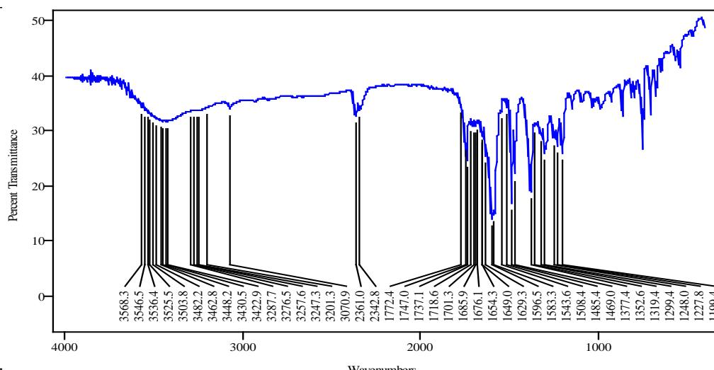
**Fig. 3: FT-IR spectra of pure ASA**
