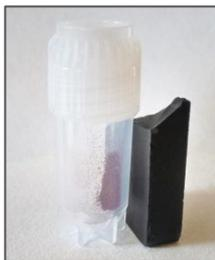
**Fig. 5: Magnetization of powder before annealing**
