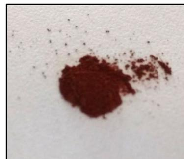
Fig. 3: Powder after annealing
