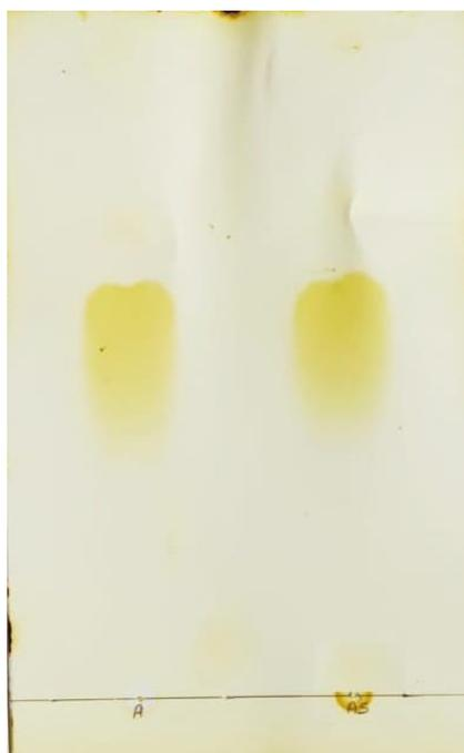
**Fig. 11: A) Thin layer chromatography (TLC) plate showing (A) Aceclofenac pure drug (B) Aceclofenac and starch malonate**
