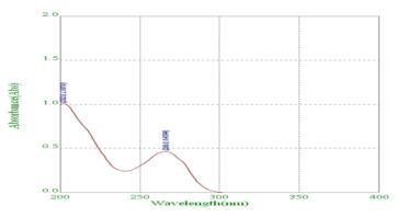
Fig. 2: UV spectrum of famotidine in phosphate buffer (pH 4.5)
