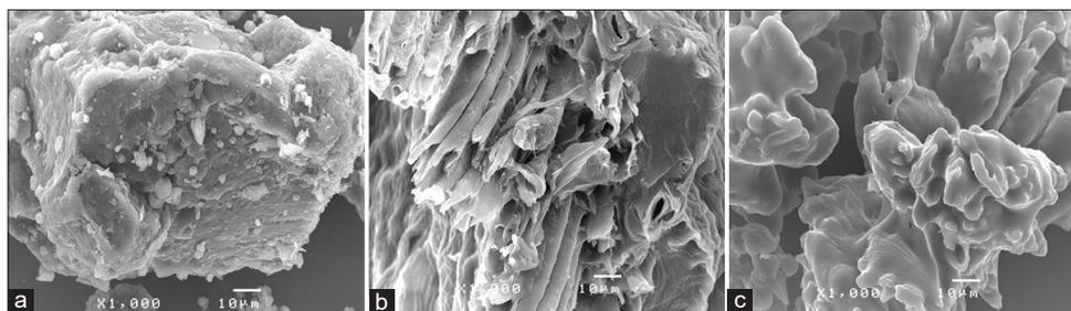
Fig. 5: Image of surface of rice husk (a), extracted cellulose (b), and extracted carboxymethyl cellulose (c) by scanning electron (magnification  $\times 1000$ )
