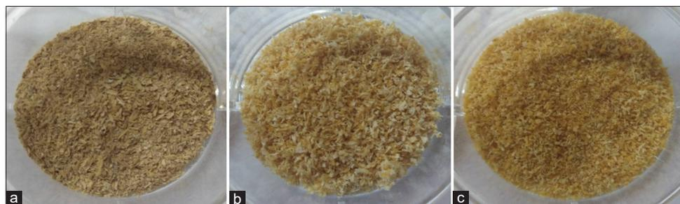
Fig. 3: Characteristics of rice husk (a), cellulose extracts (b) and carboxymethyl cellulose extracts (carboxymethyl cellulose from rice husk) (c)
