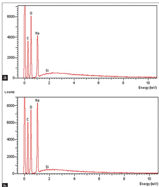
Fig. 6: Chromatogram of carboxymethyl cellulose (CMC) extracts (a) and commercial CMC (b) by energy dispersive spectroscopy
