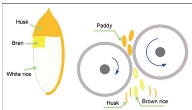
Fig. 1: The rice mill process [1]
