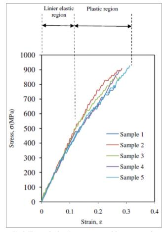
Fig. 2: The graph of strain versus stress of the sutures made from synthetic non-absorbable suture monofilament (blue polypropylene monofilament)
