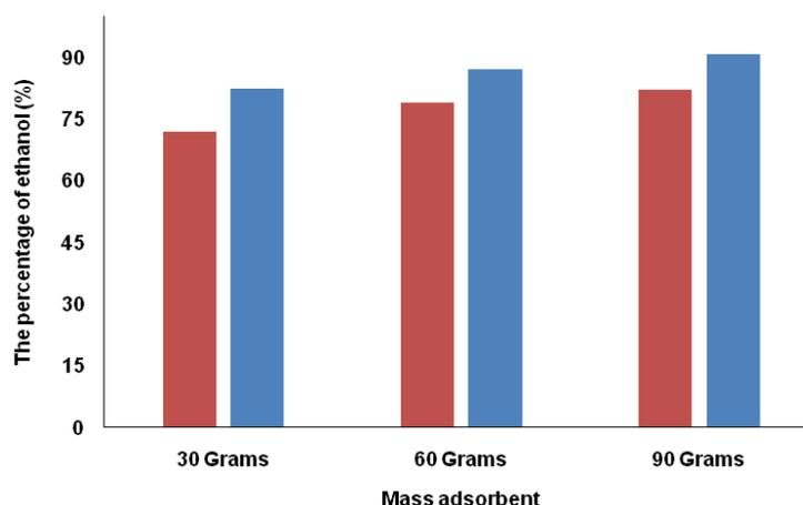
Fig. 2: Effect of mass addition of adsorbent on ethanol content orange is white silica gel and blue is synthetic zeolite 3A
