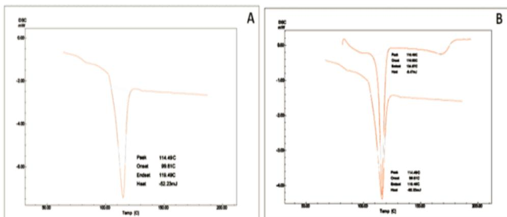
Fig. 1: DSC Thermogram; (A) Carvedilol; (B) Overlap thermogram of carvedilol and physical mixture
