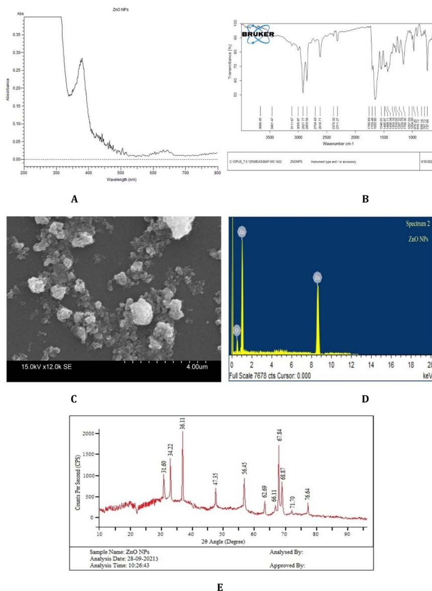
Fig. 1: Characterization of ZnO NPs synthesised using *S. swietenoides* leaf extract, A) UV-visible scanning spectra; B) FT-IR spectra; C) SEM analysis; D) EDS spectra; E) XRD analysis spectra of the synthesised ZnO NPs
