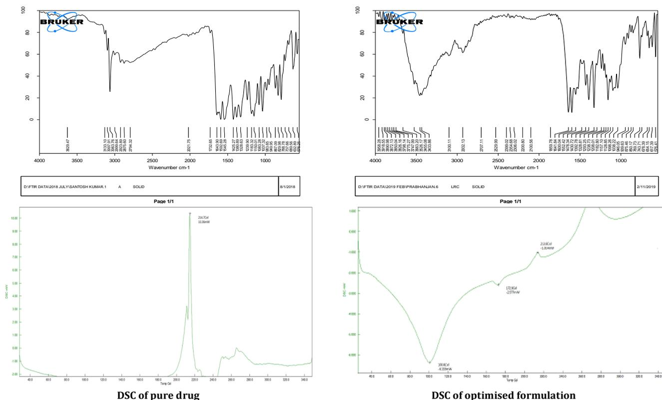
Fig. 1: The IR spectra and DSC spectra of the lornoxicam pure drug and optimized formulation
