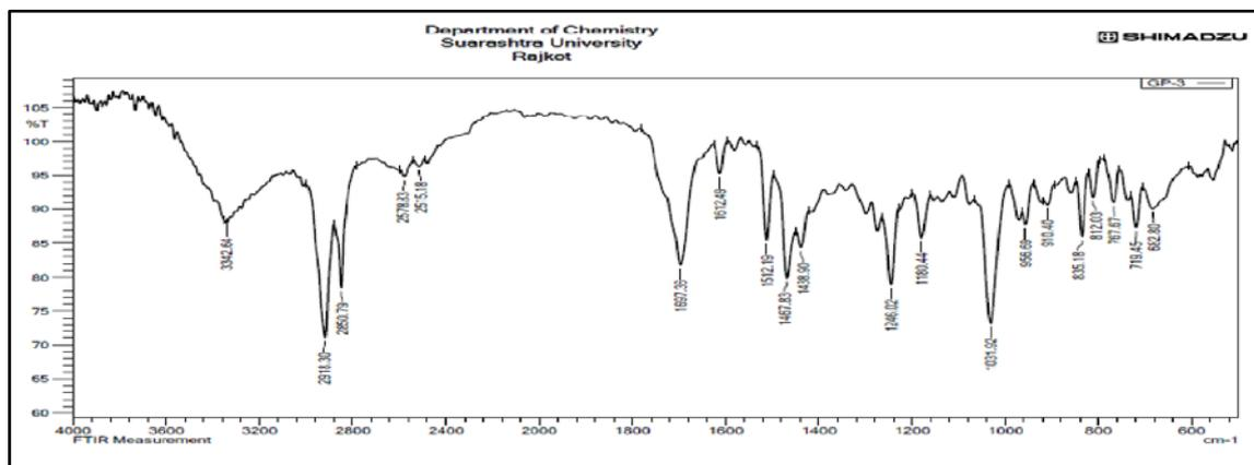
Fig. 1C: FTIR spectra of Venlafaxine HCl organogel-CR
