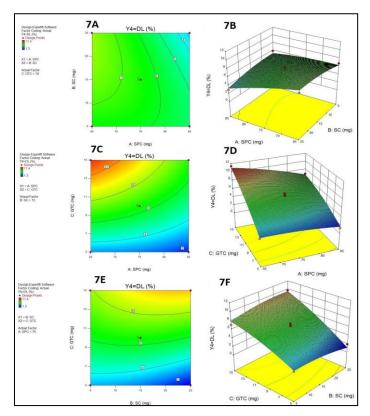
Fig. 7: Contour and response surface 3D plots showing the effects of the independent variables on DL % (Y4); two independent variables are considered at a time, while the third one remains constant. The synergistic effects (7B, 7D, 7F) of the variables on DL % are represented through the graphs
