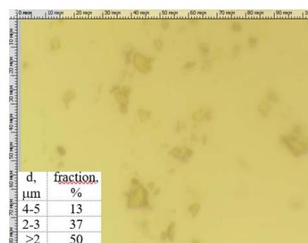
Fig. 5: Visualization of particles (size and shape) and granulometric composition (on the insert) of GAA by optical microscopy
