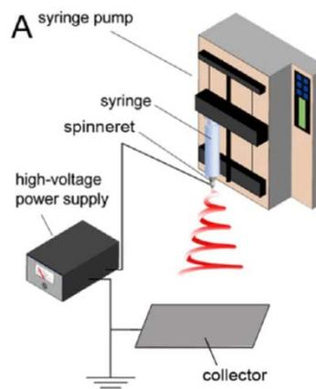
Fig. 1: Schematic illustration of a typical setup for electrospinning [15]
