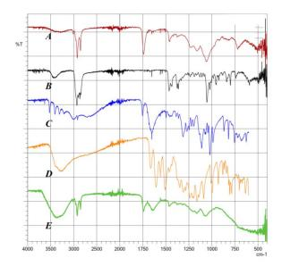
Fig. 5: FTIR spectra of soy lecithin (A), cholesterol (B), vitamin C (C), quercetin (D), and nano-phytosome sample (E)
