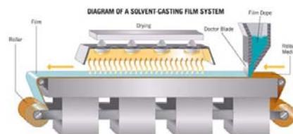
Fig. 2: solvent casting system
