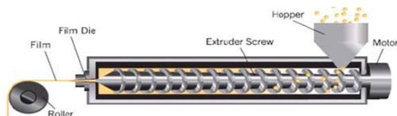
Fig. 3: Extrusion method
