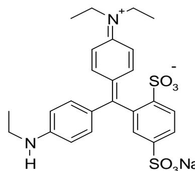
Fig. 2: Chemical structure of impurity-A (Des ethyl analogue)
