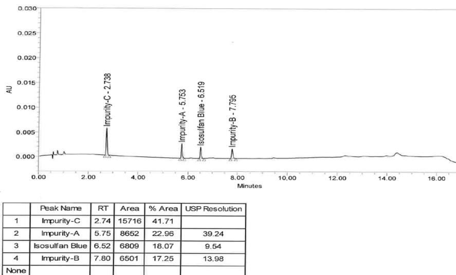
Fig. 5: Typical ultra-performance liquid chromatography chromatogram with data of system suitability (standard)
